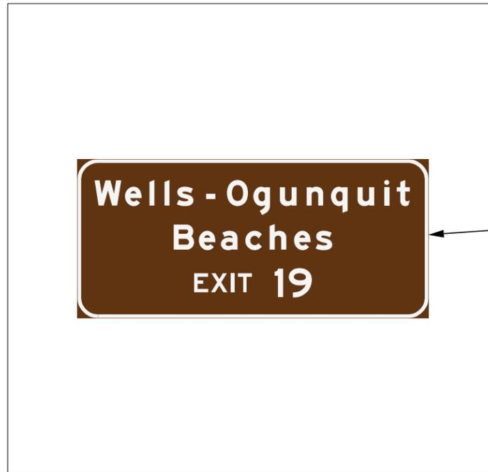
INSTALL NEW SIGN ON EXISTING SUPPORTS MOUNT TOP OF SIGN WITH TOP OF SUPPORTS
