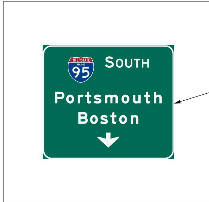
INSTALL NEW SIGN ON EXISTING CANTILEVER SIGN STRUCTURE WITH BOTTOM ALIGNED WITH ADJACENT SIGN
