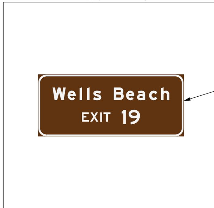
INSTALL NEW SIGN ON EXISTING SUPPORTS 2 INCHES ABOVE THE HINGE PLATE
