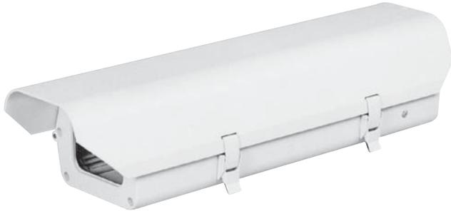
The CHG3000S Series environmental enclosures house 1/3-inch or 1/2-inch format CCD cameras. Side openings allow easy access to the removable camera sled. The weatherproof CHG3000S is designed for indoor and outdoor use and has a body length of 12.5 inches. These housings work with fixed focal length or small zoom lenses. Also available is a 24V heater/blower kit.
