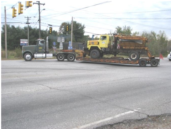
Figure 23 - Exit 75 Intersection Left turn onto Route 202/4/100. (Note: Dip below truck bed)
