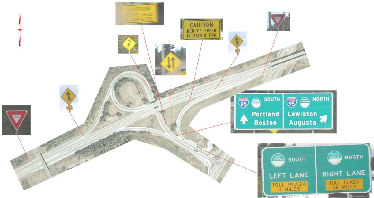
Figure 13 - Exit 75 on-ramps signing
