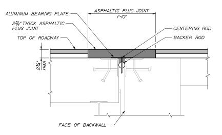
ASPHALTIC PLUG JOINT DETAIL FOREST AVENUE BRIDGE NB & SB NORTH ABUTMENT PROPOSED WORK 11/2" = 1'-0"
