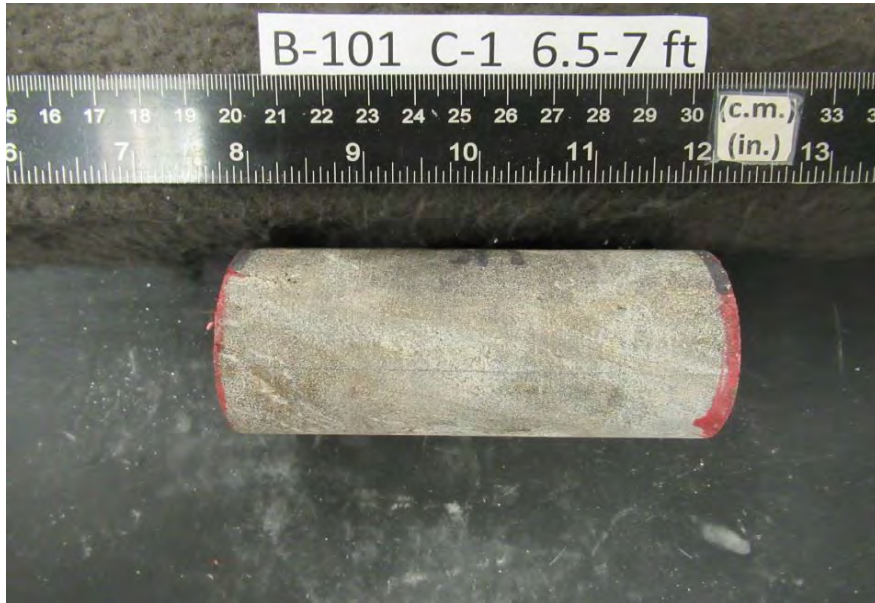
After cutting and grinding
