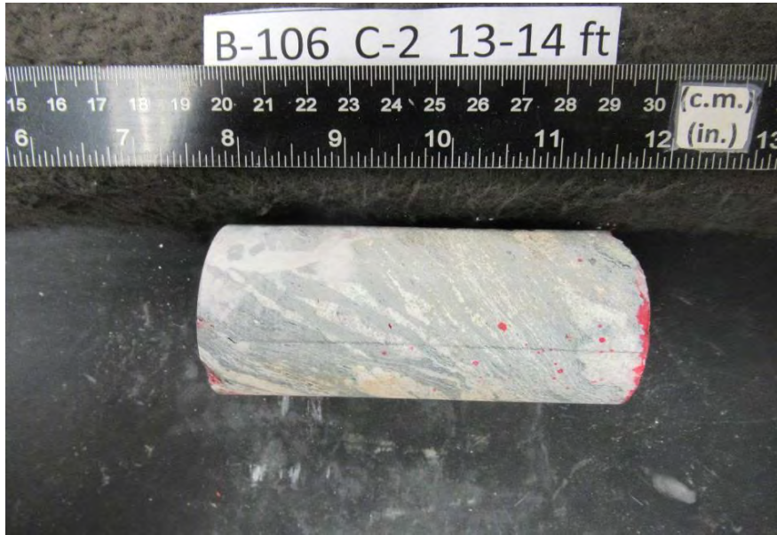
After cutting and grinding
