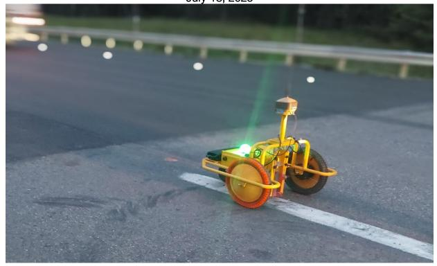
Pike currently uses a robot to assist in laying out striping on new pavement.
