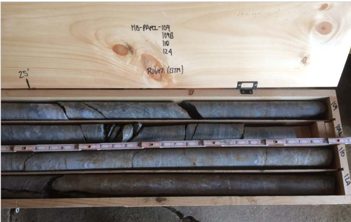
Photo 2: Core box containing dried rock core from PAMI preliminary test borings; right side of core box (bottom portion of cores). Slots from top to bottom:
