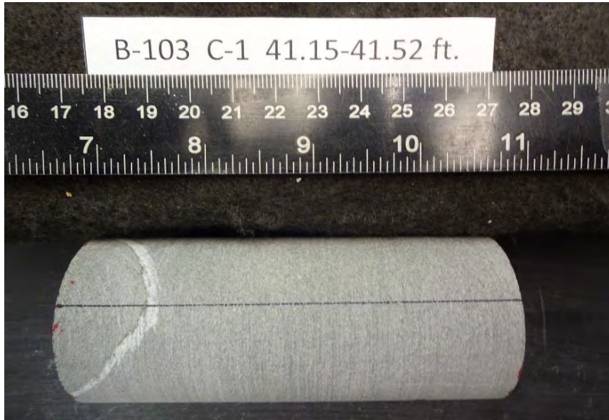
After cutting and grinding
