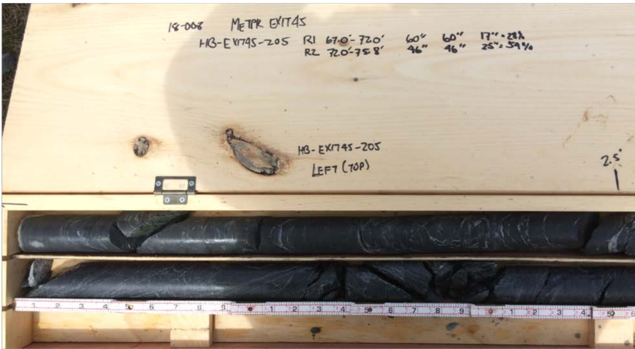
Photo 1: Core box containing wetted rock core from test boring HB-EXIT45-205 left side of core box (top portion of cores).
