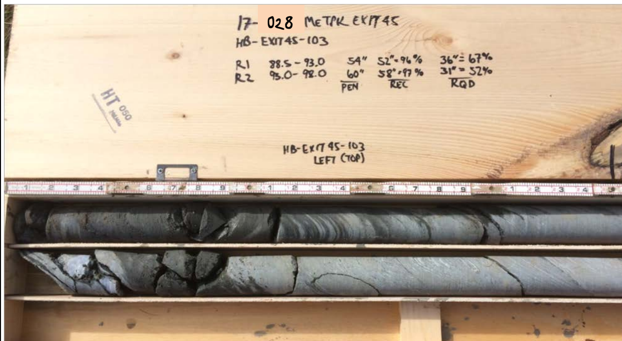
Photo 1: Core box containing dried rock core from test boring HB-EXIT45-103 left side of core box (top portion of cores).
