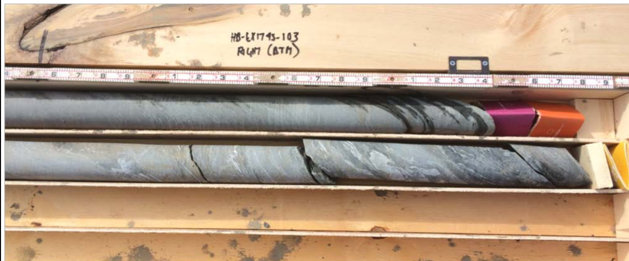
Photo 2: Core box containing dried rock core from test boring HB-EXIT45-103 – right side of core box (bottom portion of cores).
