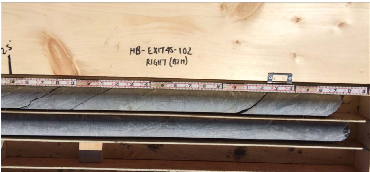
Photo 2: Core box containing dried rock core from test boring HB-EXIT45-102 – right side of core box (bottom portion of cores).
