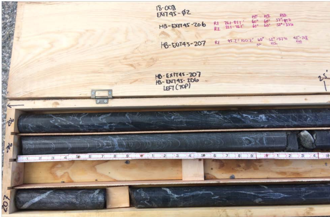
Photo 3: Core box containing wetted rock core from test borings HB-EXIT45-206 and -207 left side of core box (top portion of cores).
