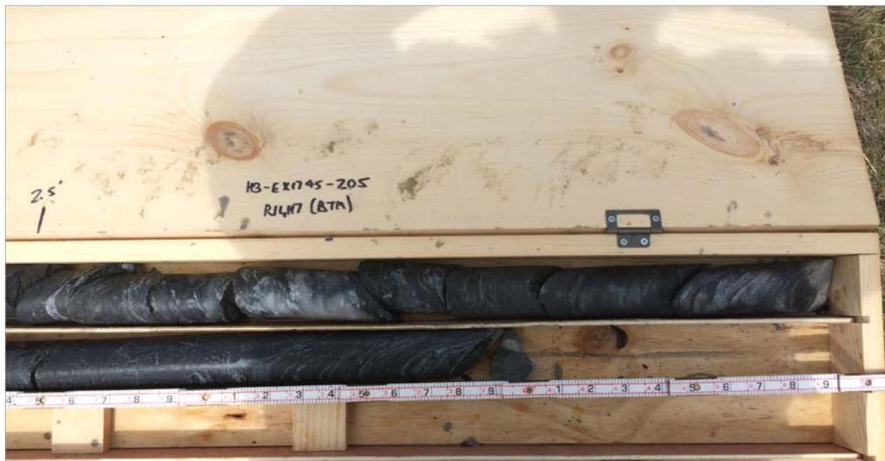
Photo 2: Core box containing wetted rock core from test boring HB-EXIT45-205 – right side of core box (bottom portion of cores).
